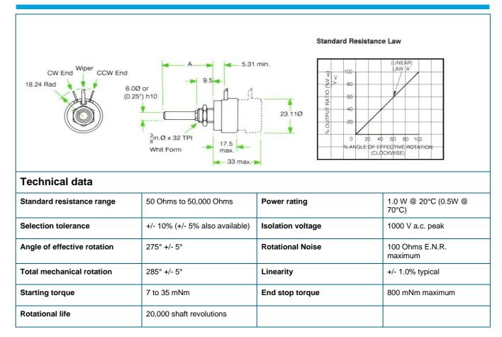
General purpose wirewound panel control of robust and reliable construction. Phenolic body moulding; beryllium copper contact; nickel plated brass spindle and bush; silver plated brass tags.
